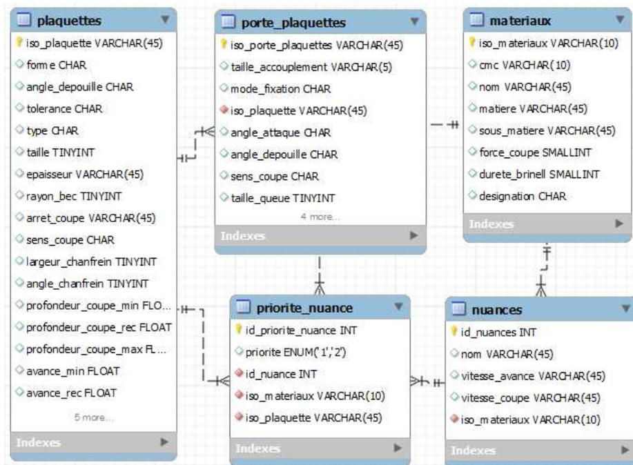
Fig. 3. Architecture of the cutting tools database
