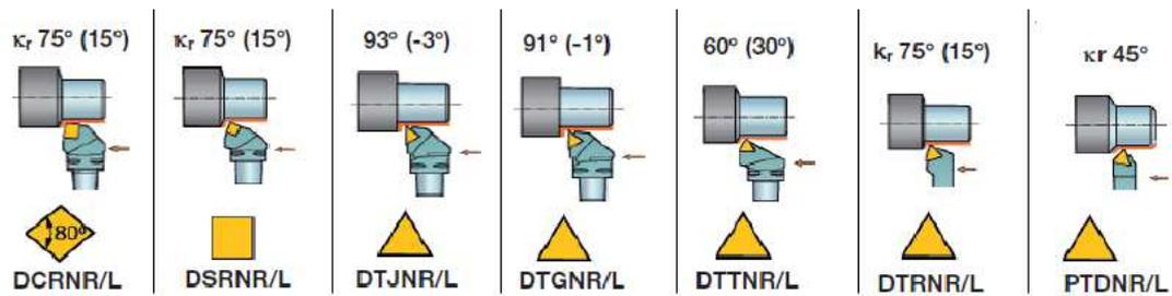
Fig. 4. Example of holders and inserts of B class of operations
