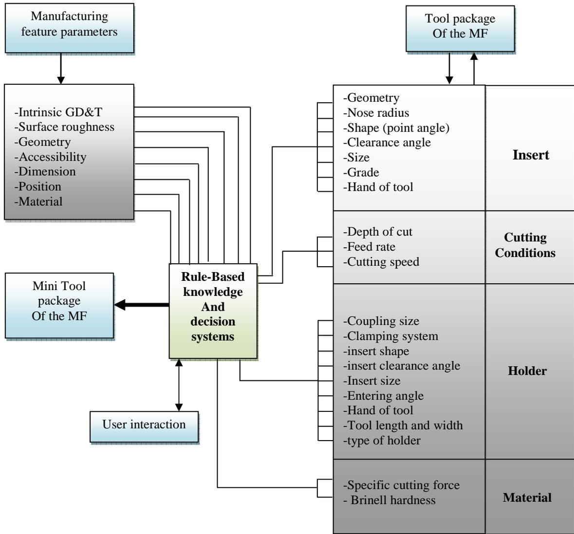
Fig. 5. Flowchart of the microscopic tool parameters choice
